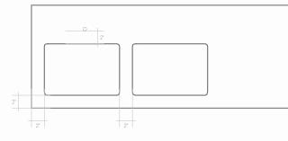
The minimum gap between a cutout and the edge of the slab must be at least 2". The size recommends distances greater than 2" when the kitchen design allows as it makes the countertop firmer
